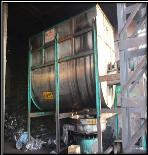
Machinery Name: 12mt Blender Location In Plant: Blender Area Capacity: 12000KGS Use: Blending Material
